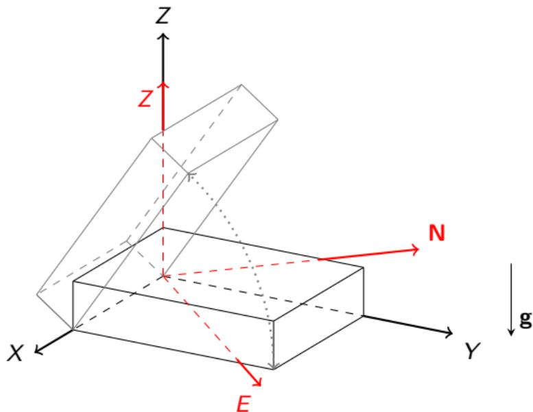
Rotate box around  $Y$  axis.
