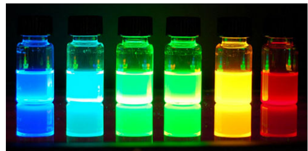
Figure 3. Photoluminescence of alloyed CdS_xSe_{1-x}/ZnS quantum dots of 6nm diameter. The material emits different color of light by tuning the composition. 7
