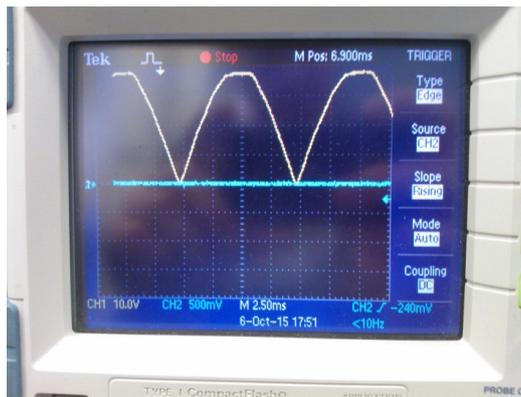
Figure 6: Full wave rectification with no smoothing
