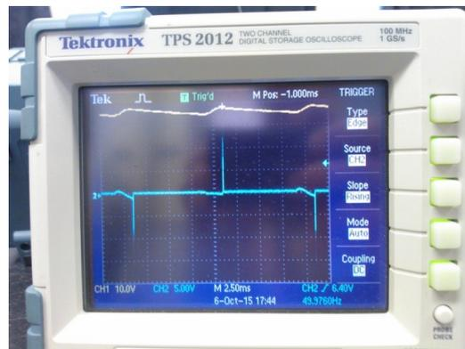
Figure 10: Smoothed output with current spike shown in blue
