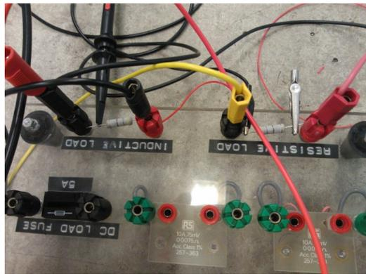
Figure 5: Showing the two 3w resistors
